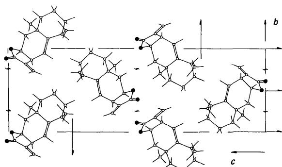
Fig. 2. The *bc* projection of the structure of alantolactone. Filled circles of the molecular models show O atoms and open circles C atoms.
